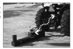
3. Attach customer supplied 3/4 inch hydraulic hose from your tractor's hydraulic supply port to the inlet port on the control valve. Connect the second hose from the tractor's return port to the outlet port on the control valve.
