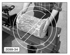
b. Using only your hand, push the control lever forward (towards the log). If the log moves before it is contacted by the splitting wedge, release the control lever and then reposition the log. Operate the log splitter only when standing in the safe operating area, as shown in the picture.
