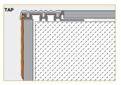
**Schluter®-TREP-TAP** is an anodized aluminum cover profile that integrates with the Schluter®-TREP-S/-B stair-nosing profiles to conceal the top of the riser.
