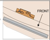
8. Install the mounting screw half way through the bracket attached to the top of the recess box. (Figure 4)
