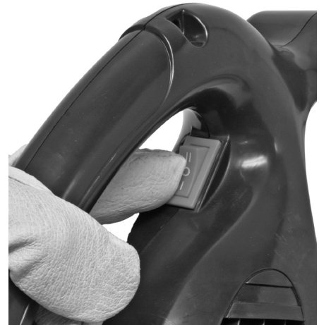
Figure 4-6: On/Off Switch to LOW position
