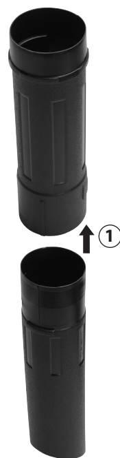
Figure 3-8: Connecting lower and upper vacuum tube together
