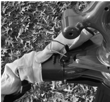
Figure 4-10: Removing bag/adapter assembly
