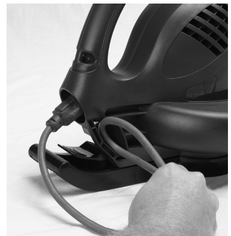
Figure 4-2: Inserting extension cord loop through cord slot
