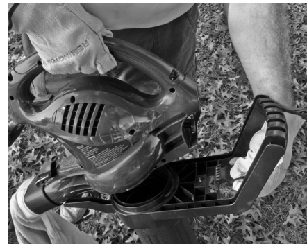
Figure 4-13: Removing vacuum tube adapter
