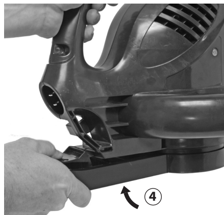
Figure 3-4: Pivoting bottom inlet cover to blower/vac housing
