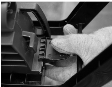
Figure 4-12: Pressing locking lever
