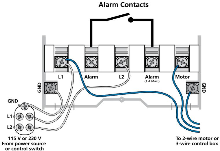
**Figure 3: Wiring Connections**
