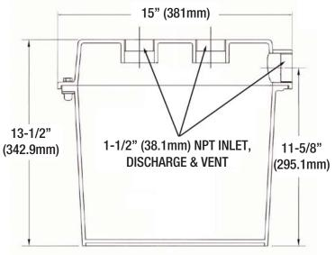
\* All measurements are nominal. Please verify before actual installation. DO NOT USE WITH AN AUTOMATIC AIR ADMITTANCE VALVE.
