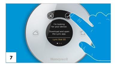
Your thermostat will light up while it starts up - this may take up to 3 minutes. When the thermostat stops, it will display a unique network name, for example, Lyric Stat O3. When you see the unique network name, touch "OK" to begin your thermostat configuration.
