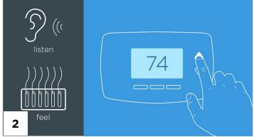
**Verify the power is off.** Go to your thermostat and try increasing or decreasing the temperature. Many digital thermostats are battery powered, which makes it difficult to tell if the power is off. Listen to ensure your system is turned off before continuing.
