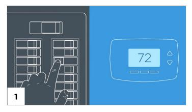
**Switch off the power** to your heating and/or cooling system at the circuit breaker box or at the system switch or on your heating and/or cooling unit.
