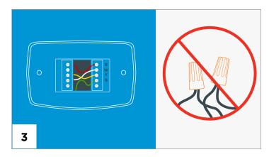
Remove the front of the old thermostat but keep the wallplate with wires attached. Check the wires to see what type of voltage you have. Do you have thick black wires with wire nuts? Is your thermostat 110 volts or higher? If yes, you have a line voltage system, and the Lyric thermostat will not work. For more options, please visit yourhome.honeywell.com/home/Products/Thermostats
