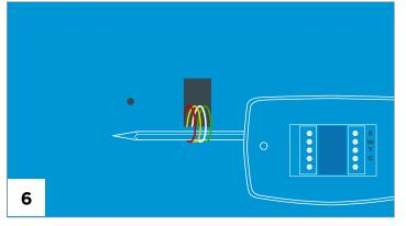
Once all wires have been recorded, **disconnect them** from your old thermostat. **Remove the old wallplate from the wall.** To prevent wires from falling back into the wall, wrap the wires around a pencil.
