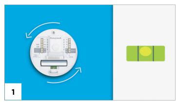
After threading the wires through the wallplate, mount the wallplate of the Lyric thermostat. Make sure it's level by verifying the bubble of the self-contained level is between the two lines. (Included in the box is an optional trim ring you can use to cover wall blemishes. If you choose to use the trim ring, attach it to the wallplate prior to mounting.)
