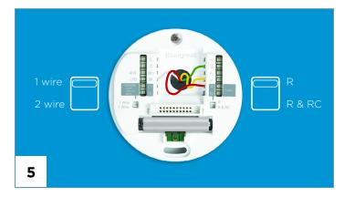
Your app will also tell you whether the **slider tab on the left and right of the wallplate** needs to be pushed up or down based on your R-wire installation. If your old thermostat had only one R-wire connected, make sure the slider tab is pushed up to cover the RC connection. If your thermostat has two R-wire connections, R and RC, push the slider tab down.
