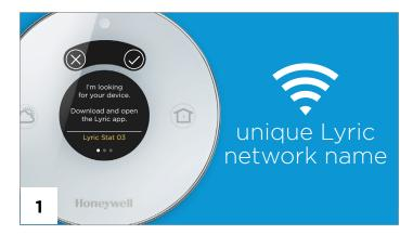
**Connect your smartphone or tablet to the thermostat network.** Your new thermostat should be displaying a unique network name, such as Lyric Stat 03.
