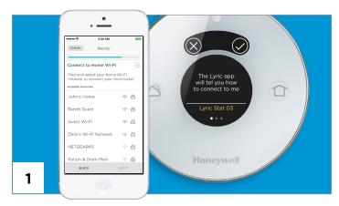
From the Lyric app, select your Wi-Fi network to connect your thermostat (or manually add it). Enter your password if password protected. The thermostat is now connecting to your home Wi-Fi network. It will take up to three minutes to establish a connection and sync with Honeywell. (During this time, do not navigate away from the Lyric app.) If an error appears on your thermostat screen, touch "Connect Again" to re-establish the connection.
