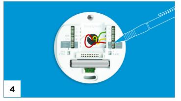
To insert wires, slide each wire into its corresponding terminal and ensure it is secure by gently tugging.
