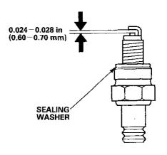
6. After the spark plug seats, tighten with a 5/8-inch spark plug wrench to compress the washer.
