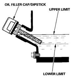
4. Screw in the oil filler cap/dipstick securely.
