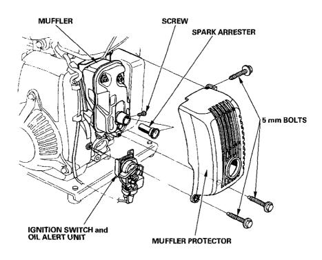
3. Use a brush to remove carbon deposits from the spark arrester screen. Be careful to avoid damaging the screen.
