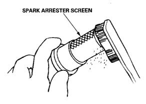
4. Install the spark arrester and the muffler protector in the reverse order of disassembly.
