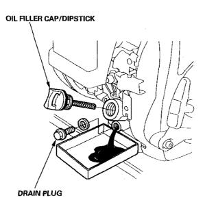
3. With the engine in a level position, fill to the edge of the oil filler hole with the recommended oil (see page 33).
