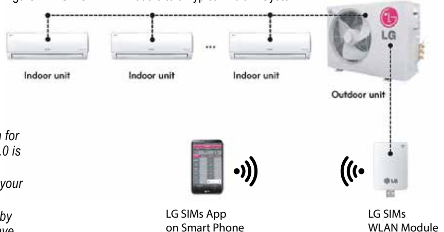
Figure 71: SIMs WLAN Module to a Typical Multi F System
