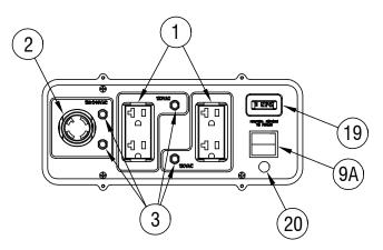
Figure 2B - Control Panel (CARB Models)
