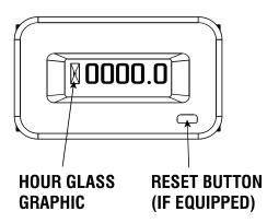
When the hour meter is in the Flash Alert mode, the maintenance message will always alternate with elapsed time in hours and tenths. The hours will flash four times, then alternate with the maintenance message four times until the meter resets itself.
