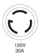
Use this receptacle to operate 120 Volt AC, 60 Hz, single phase loads requiring up to 3600 watts (3.6 kW) of power at 30 Amps. The outlet is protected by a 30 Amp push-to-reset circuit breaker.
