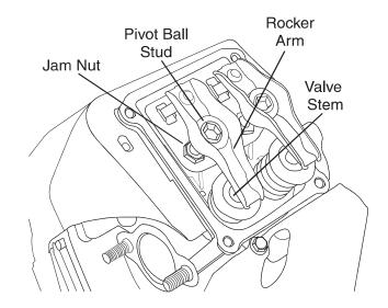
When valve clearance is correct, hold the pivot ball stud in place with the allen wrench and tighten the rocker arm jam nut. Tighten the jam nut to 174 in/lbs. torque. After tightening the jam nut, recheck valve clearance to make sure it did not change.
