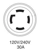
Use this receptacle to operate 120 Volt AC, 60 Hz, single phase loads requiring up to 3600 watts (3.6 kW) of power at 30 Amps or 240 Volt AC, 60 Hz, single phase loads requiring up to 7200 watts (7.2 kW) of power at 30 Amps. The outlet is protected by two 30 Amp push-to-reset circuit breakers.
