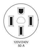
Use this receptacle to operate 120/240 Volt AC, 60 Hz electrical loads requiring up to 12,000 watts (12.0 kW) of power. This receptacle is protected by a 50 Amp 2-pole circuit breaker.
