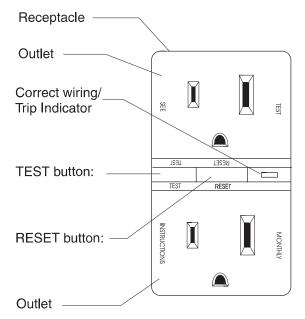
Testing the GFCI: Test the GFCI outlet every month as follows:
