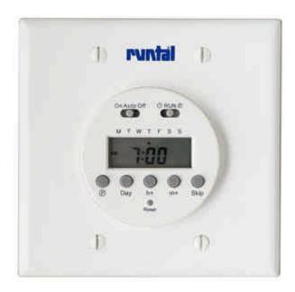
The Electric Programmable Controller (EPC) may be used with all electric towel radiators. It fits into a double-gang box and provides seven day individual programming with up to eight different ON/OFF cycles per day. Use the Programmable Controller to provide a warm bathroom first thing in the morning; to avoid heating the rest of the house in the spring and fall; and to provide comfortable heat and warm towels to meet everyone's daily routine.
