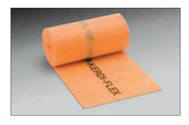
**KERDI-FLEX** is a flexible polyethylene waterproofing strip used to seal movement joints over DITRA in specialty applications where large movements are expected, i.e. over expansion joints or construction joints.
