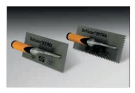
Used to install DITRA and KERDI membranes. The **DITRA-TROWEL** features an 11/64" x 11/64" (4.5 mm x 4.5 mm) square-notched design while the **KERDI-TROWEL** features a 1/8" x 1/8" (3 mm x 3 mm) square-notched design.
