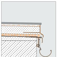
Schluter products make it easy to construct functional balcony coverings that include subsurface drainage, uncoupling/waterproofing, tightly sealed wall joints, and gutters.
