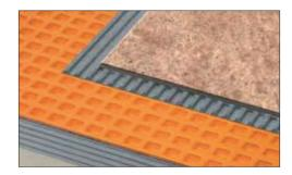
**DITRA-XL** is a pressure-stable polyethylene membrane, vacuum-formed in a cutback grid design, with an anchoring fleece laminated to its underside. DITRA-XL is 5/16" (7 mm) in height and emits zero VOC.
