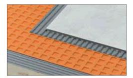
**DITRA** is a pressure-stable polyethylene membrane, vacuum-formed in a cutback grid design, with an anchoring fleece laminated to its underside. DITRA is 1/8" (3 mm) in height and emits zero VOC.
