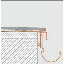
Balcony assemblies with waterproofing, integrated gutter, and waterproof wall connections can easily be built using Schluter products, as indicated.
