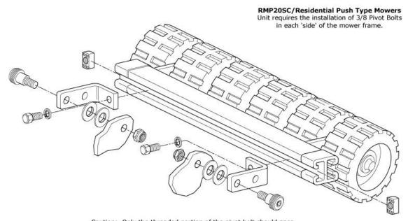
Caution: Only the threaded portion of the pivot bolt should pass through the mower frame. If mounting in oversize hole, please use 3/8" flat washer on both inside & outside of frame to prevent smooth portion of pivot bolt from passing through mower frame.
