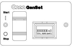
FIGURE 1-5. REMOTE SWITCH / HOUR METER
