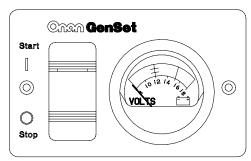
FIGURE 1-6. REMOTE SWITCH / DC VOLTMETER
