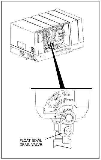
FIGURE 2-3. CARBURETOR DRAIN VALVE (GASOLINE MODELS ONLY)
