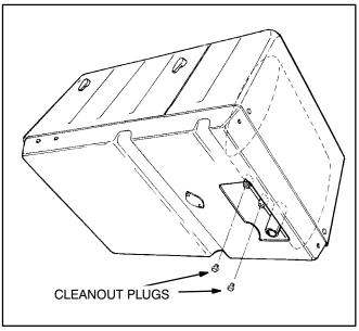
FIGURE 3-5. SPARK ARRESTOR CLEANOUT PLUGS
