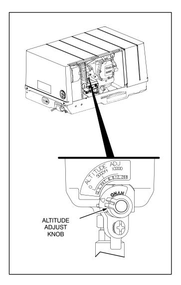
FIGURE 2-2. ALTITUDE ADJUST KNOB (GASOLINE MODELS ONLY)
