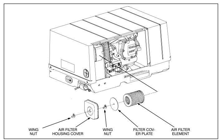
FIGURE 3-3. REPLACING THE AIR FILTER ELEMENT
