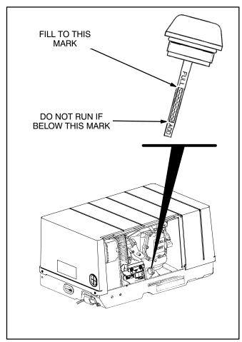
FIGURE 3-1. CHECKING ENGINE OIL LEVEL
