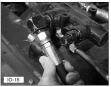
15. Coat the threads of the fitting with a hydraulic pipe sealant and attach the high-pressure hose from the bottom valve fitting to the pump, as shown. Securely tighten the hose fitting.
