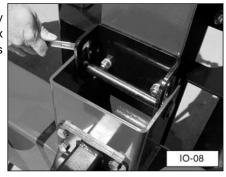
7. Bolt the rail rest to the rail assembly using two 1/2-13 x 1-1/2 inch long hex head bolts, lockwashers, and nuts, as shown. Hand tighten the nuts.
