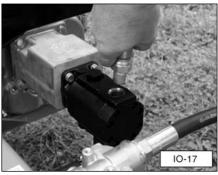
16. Remove the oil filter from the plastic cover and apply a thin coat of oil to the rubber seal. Screw the filter onto the filter head located near the hydraulic tank. Once the filter makes contact with the filter head, turn it an additional 3/4 turn. Hand-tighten only.
