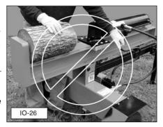
c. Hold the control lever, extending the splitting wedge, until the log is split or the cylinder rod stops at its maximum travel position. Stop the log splitter (forward movement) at any point in the splitting process if you feel an unsafe log splitting condition is occurring. As the log is being split, DO NOT reach forward and attempt to catch the split wood — let it fall to the ground.
