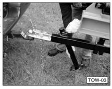
**4.** Place a customer supplied lock or lock pin into the latch assembly of the hitch coupler.
