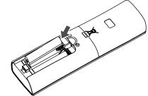
Figure 5: Battery Placement
