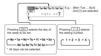
(3) Press  $\bigcirc$  (0)/OFF, time, and  $\square$  buttons to set ON/OFF, time, and temperature.
