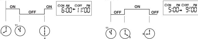
**NOTE:** If the main power is turned OFF or a power failure occurs while ON/OFF timer is active, the timer setting is cancelled. As these models are equipped with an auto restart function, the air conditioner starts operating with timer cancelled when power is restored.
