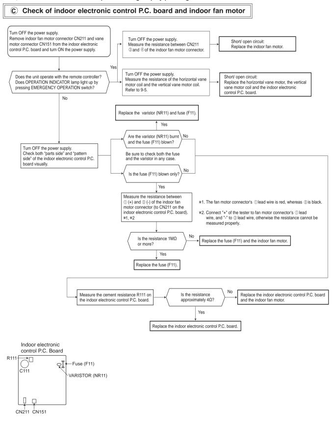
When the left lamp of OPERATION INDICATOR lamp flashes ON and OFF in every 0.5-second. Outdoor unit does not operate.
