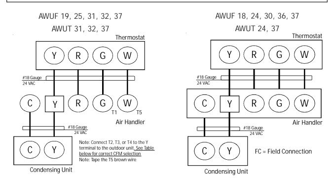
NOTE: Connect appropriate speed tap (Pink/Purple/Yellow) to Y. Refer to table below for speed tap selection. It is not recommended to use the 1 Ton application for AWUF19 8kW heater models.
