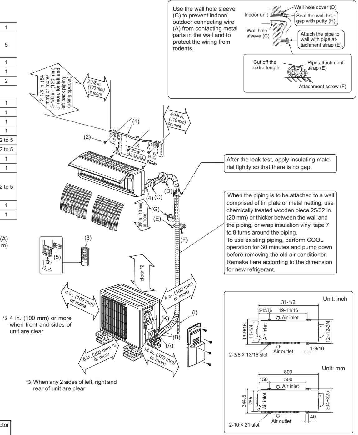
After the leak test, apply insulating material tightly so that there is no gap.
