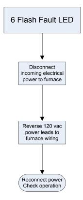
DEFINITION: External Gas Valve Circuit Error (24 volts is present when it should not be present)
