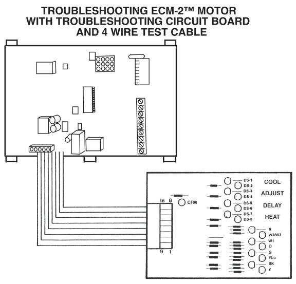
**Purpose:** Verify proper signals are being received by the motor control board and are being sent to the ECM-2<sup>™</sup> Motor by the 16 wire low voltage motor harness.
