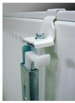
When hanging radiator onto brackets, Set the backside bottom onto lower hook, Then latch the top onto the top grill.
