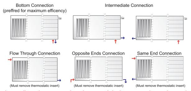
Note: when installing radiators in series/loop it's reccomended to have no more than 3 radiators in line.
