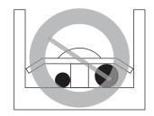
On not terminate different gauge wires to a terminal block.
