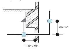
Figure 32: Pipe Support at Indoor Unit.
