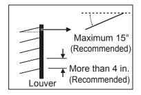
Figure 9: Using "S" Type Louvers.
