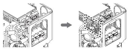
Figure 94: PI-485 Board (Appearance will differ depending on model).
