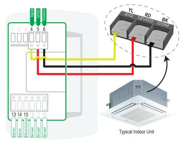
Figure 97: Another Example of Indoor Unit to Zone Controller Connection.
