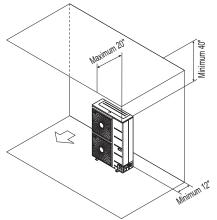
Obstacles above, on the air intake side, and on both left and right sides.
