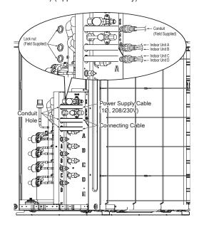
Figure 89: Connecting the Power Wiring / Communications Cables to the Outdoor Unit (LMU483-543HV).
