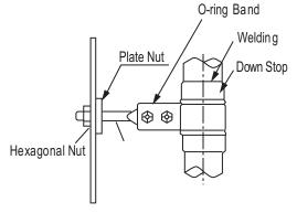
Figure 41: Two-Point Down-Stop Support.
