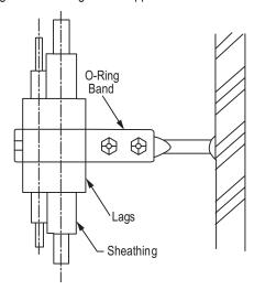
Figure 40: One-Point Down-Stop Support (>441 lbs.).
