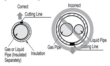
Figure 69: Piping with Insulation Material.
