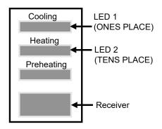
Figure 132: Example of Art Cool Mirror Wall-Mounted Indoor Unit LEDs.
