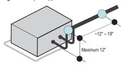
Figure 33: Pipe Support at Y-branch Fitting.
