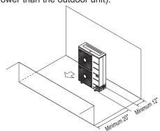
Where there are obstacles above, and on both suction and discharge sides (discharge side obstacle
