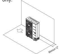
Obstacles on the suction side and on both left and right sides.
