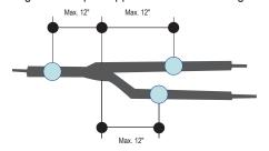
Figure 34: Pipe Support at Header Fitting.
