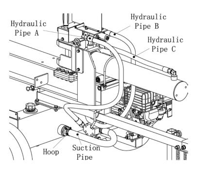
Step 6: Attach control valve to cylinder
