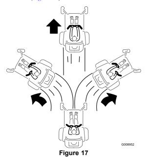
To go straight, apply equal pressure to both motion-control levers (Figure 17).
