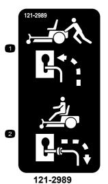
Bypass lever position for pushing the machine
