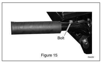
20. Position the trigger beneath the right side handlebar. Insert 1/4" machine screw (item 21) through the 1/4" internal locking washer (item 20). Insert the 1/4" machine screw (item 20) through the handlebar in the place of the bolt removed in Step 19. Thread the screw (item 21) into the trigger to attach it to the machine. See Figure 16.
