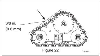
If unit pulls to the left or right when a straight path is desired adjust the track tension. If the unit is pulling to the left, tighten the left track adjuster. If the unit is pulling to the right, tighten the right track adjuster.
