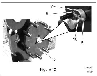
Apply anti-seize compound or waterproof grease to the left axle shaft and install track drive wheel (item 2) onto shaft. Install 5/8" snap clip (item 13) to end of axle. See Figure 13.
