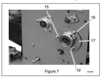
10. Lift the carriage assembly (item 1) into position around the frame with the adjustable axle toward the rear of the unit. Align the bearings on the frame to the bearings on the track carriage and place the spacer (item 19) between the two bearings. Insert the short axle (item 3) into the right side flange bearing, being careful not to push out bushings. See Figure 8 and Figure 18.
