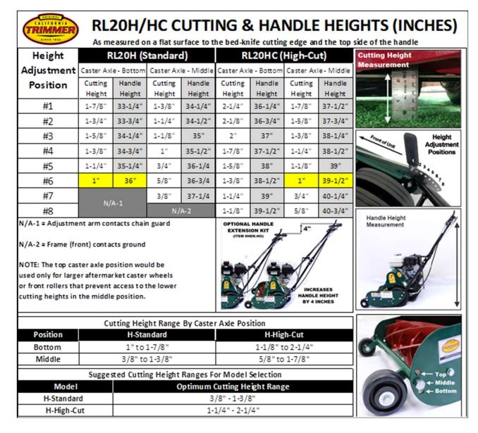
The Handle Extension kit adds about 4" to the overall height of the handles and is typically preferred by people 6' 2" and taller... especially on the Standard models – as the High-Cut models are already about 2" higher at the handles.
