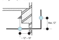
Figure 42: Pipe Support at Indoor Unit.
