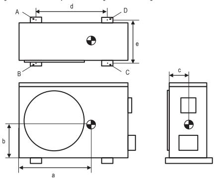
Table 6: Center of Gravity and Corner Weight Dimensions.
