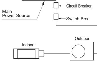
Figure 48: Power Wiring Example
