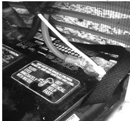
Figure 3.17 - Reconnect Battery Cables.
