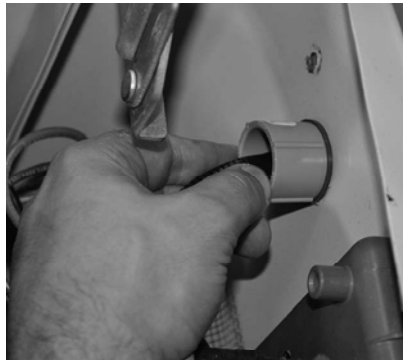
Figure 3.7 - Installing Fitting with Harness
