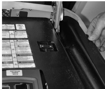
Figure 3.3 - Removing Controller Fascia
