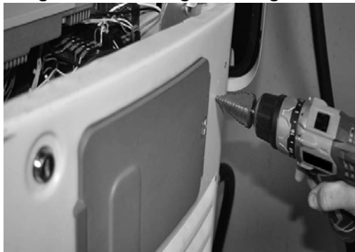
Figure 3.5 - Drilling Mounting Hole.
