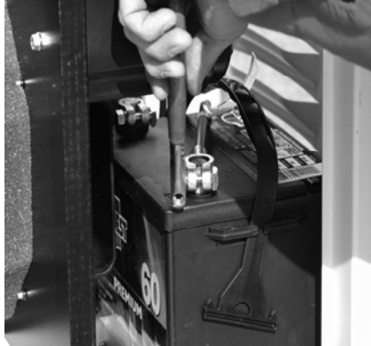
Figure 3.2 - Removing Battery Cables
