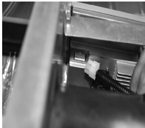
Figure 3.15 - Harness Installed to Controller.
