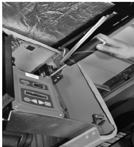
Figure 3.13 - Removing Controller Fasteners.
