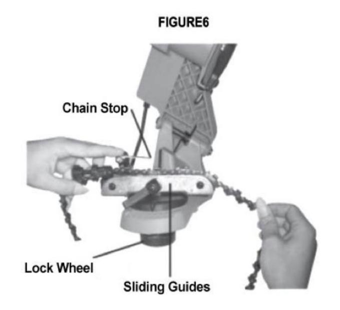
3) Lower the chain stop so that it's positioned on the tooth (blade) you want to start with.
