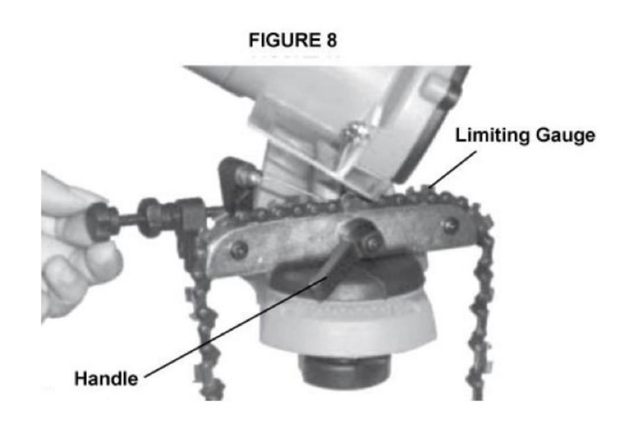
9) If the chain has been repeatedly sharpened, the chain depth limiting the gauges may need to be taken down with a flat file (not included). File down each gauge so that they are at a lower level than the cutting teeth.
