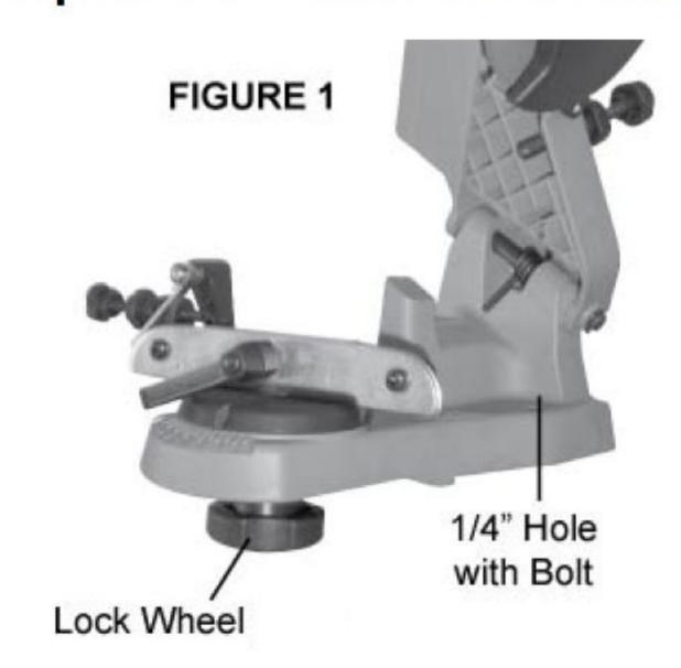
2) Bolt the unit directly to the workbench through the two 1/4in holes on the base (bolts not included). The workbench must have a solid surface that is capable of supporting the weight of the sharpener, tool and work pieces.
