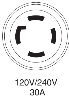
Figure 7 - 120/240 VAC, 30 Amp Receptacle
