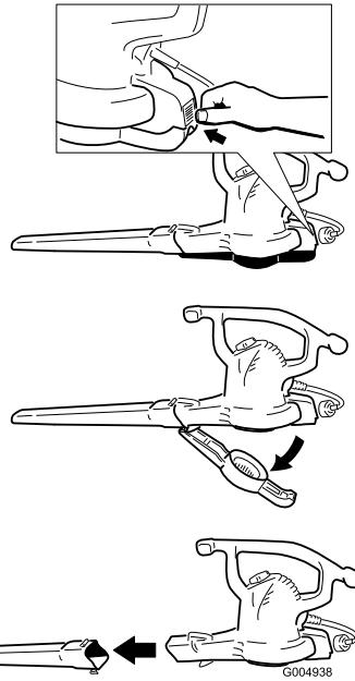
2. Install the vacuum tube onto the blower housing.
