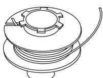
3. Wind the line in the direction of the arrow on the spool, in level rows, between the spool flanges.
