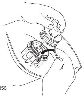
2. Holding the line and spool, place the cap over the spool.
