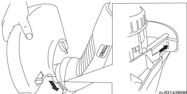
2. Snap the guard into place and secure the hooks under the guard on to the trimmer.
