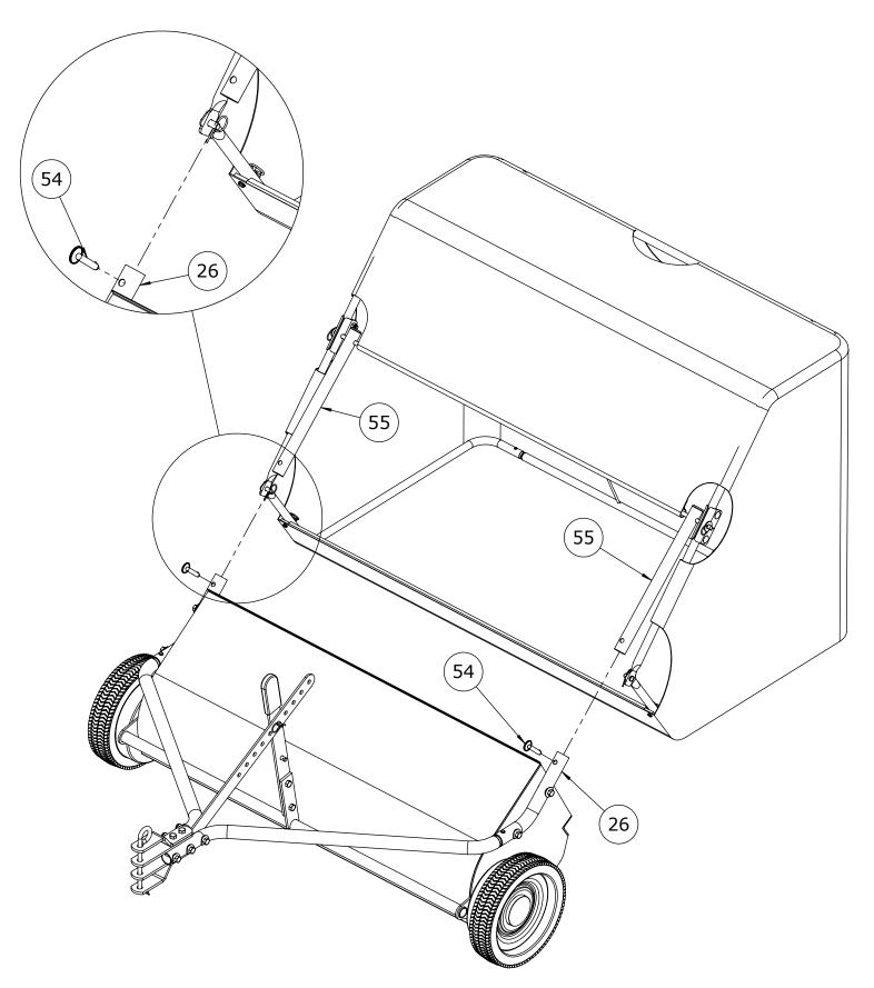
Step 10. Insert hopper connect tubes (55) into hitch mount tubes (26) as shown and lock in place with 3/8" ring grip pins (54).
