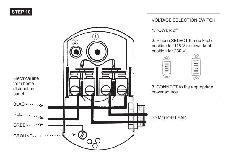
We recommend that a licensed electrician be employed to do wiring to the pressure switch. Permanently ground the motor in accordance to the electrical codes for your area.
