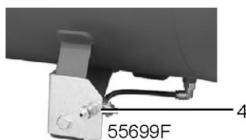
Condensate drain valve on air receiver
