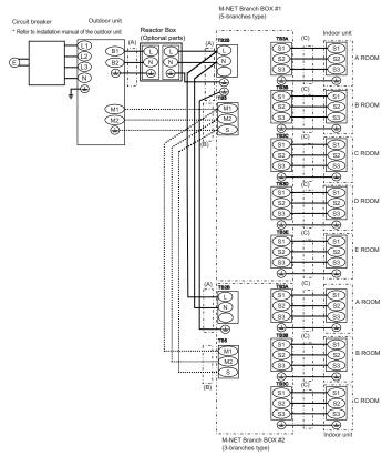
© Power supply: Single phase 220/230/240 V 50 Hz, 220 V 60 Hz
