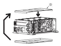
$\ensuremath{ \bigcirc \!\!\! /}$  Install the electric cover on the opposite surface.  $\ensuremath{ \bigcirc \!\!\!\! /}$  Electric cover
