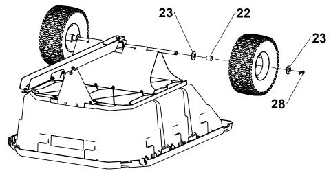
6 Install Hitch Pin as shown.
