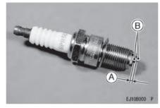
A. Spark Plug Gap B. Electrodes
