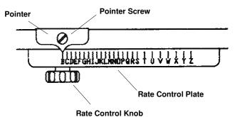
2. Flip on/off control lever to the "ON" position. Check the port opening. It should be just open. If adjustment is necessary, continue to step #3.
