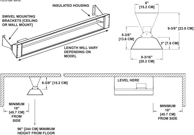
Heater must be installed with the Quartz horizontally level. For maximum tube life, use a carpenter's level tool to find the optimum level position for the heater's body. Always maintain the minimum clearances from the heater body to any combustible materials.
