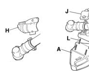
Remove the mounting plate (H). Fit the adapter (I) and bracket (J) with the two screws (K) as shown. Fit the blade guard (A) to the adapter using the 4 screws (L) as shown.
