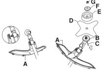
Hook the blade guard/combination guard (A) onto the fitting on the shaft and secure with the bolt.
