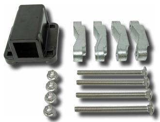
The DHRUM mounting kit can be used to mount your DHRTM50200 trailer mount hose reel to a wall or a wide range of portable pressure washer frames. The clamp system securely attaches to any round pipe or square tube frame up to 2" in size/diameter. The clamps grip to the frame to prevent slippage. The bracket consists of one powder-coat & rust-proof aluminum receiving socket, four galvanized steel clamps, and four stainless steel nuts and bolts.
