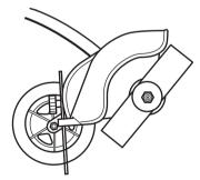
Check that the guard is undamaged and not cracked. Replace the guard if it has been exposed to impact or is cracked. Always use the recommended guard for the cutting attachment you are using. See chapter on Technical data.
