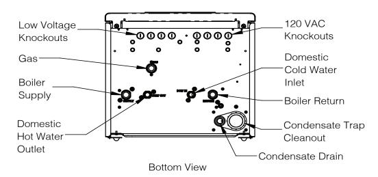
Figure 3-6: Boiler Connections
