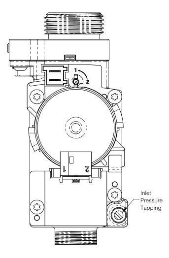
Figure 15-8: Gas valve inlet pressure tap
