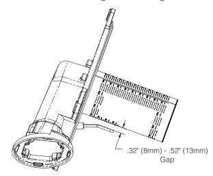
Figure 18-3: Ignitor/flame sensor to burner gap
