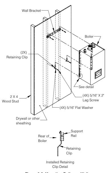
Figure 6-5: Mounting Boiler on Wall
