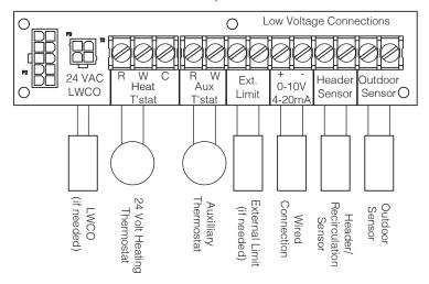
Figure 13-3: Low Voltage Connections
