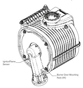
Figure 18-1: Ignitor/flame sensor location
