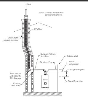
Figure 9-16: Masonry Chimney Chase System
