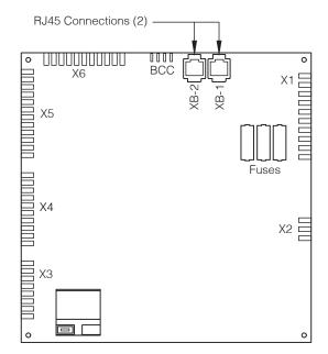
Figure 13-4: Boiler Peer-to-Peer Connections
