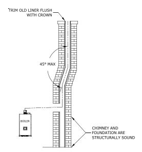
Figure 9-17: Masonry Chimney Chase Requirements
