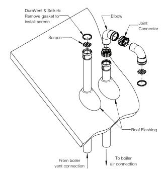
Figure 9-4: Polypropylene Fittings Terminal Assembly
