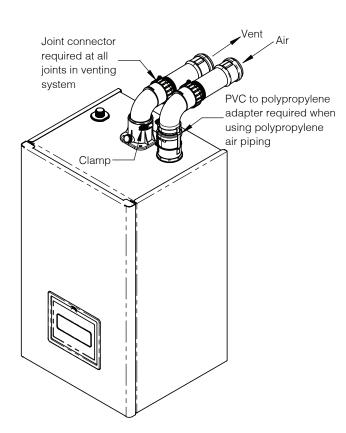
Figure 7-18: Near Boiler Polypropylene Venting
