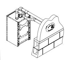
Figure 7-2: Sidewall Low Profile Termination - see Section 8 for details
