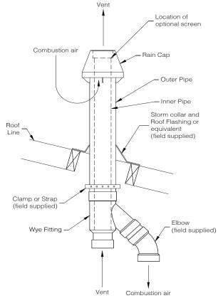
Figure 9-7: CPVC/PVC Concentric Vertical Installation
