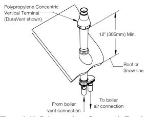
Figure 9-10: Polypropylene Concentric Terminal
