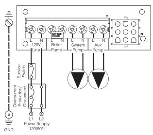
Figure 13-2: 120 VAC Connections
