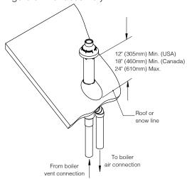
Figure 9-6: CPVC/PVC Concentric Terminal
