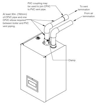
Figure 7-12: Near Boiler CPVC/PVC Venting
