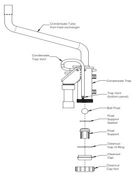
Figure 18-4: Condensate Trap Exploded Parts View
