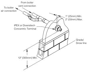
Figure 8-10: CPVC/PVC Concentric Terminal
