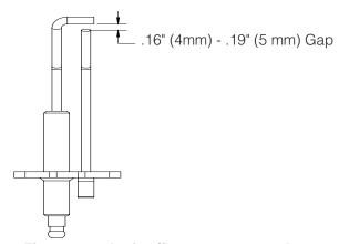
Figure 18-2: Ignitor/flame sensor spark gap
