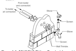
Figure 8-5: CPVC/PVC Fittings Terminal Assembly
