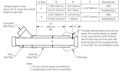
Figure 8-12: CPVC/PVC Concentric Terminal Dimensions
