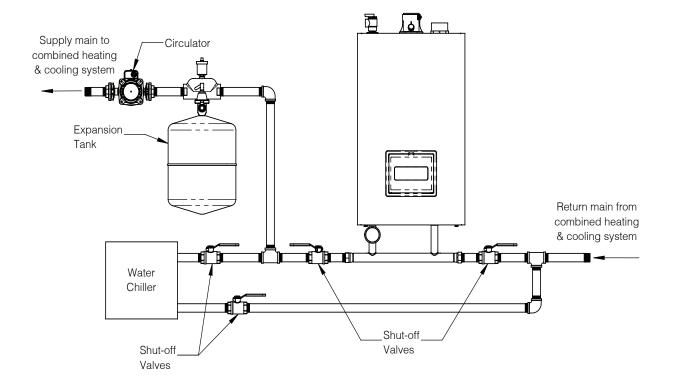
Figure A-1: Isolated Boiler from Refrigeration System
