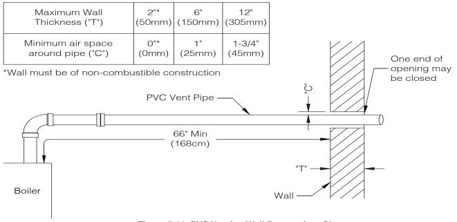
Figure 7-14: PVC Venting Wall Penetration Clearance
