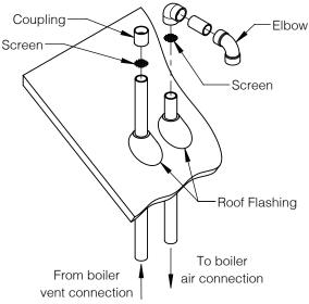
Figure 9-3: CPVC/PVC Fittings Terminal Assembly
