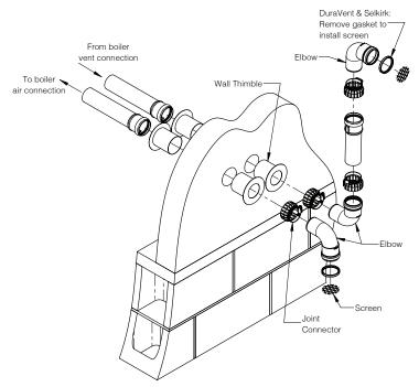
Figure 8-6: Polypropylene Fittings Terminal Assembly
