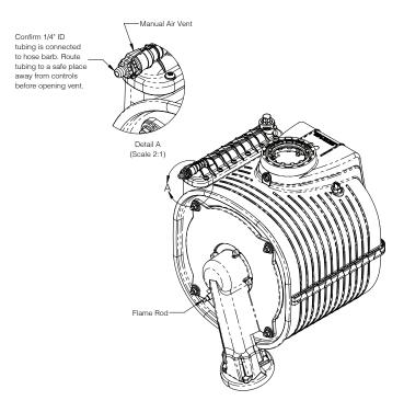
Figure 15-1: Manual Air Vent Location
