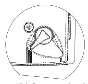
Figure 15-2: Pump speed setting
