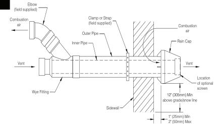
Figure 8-11: CPVC/PVC Concentric Terminal Installation
