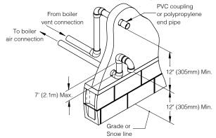
**Figure 8-4: Alternate Fittings Terminal**
