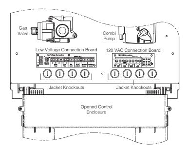
Figure 13-1: Location 120VAC and low voltage connection boards
