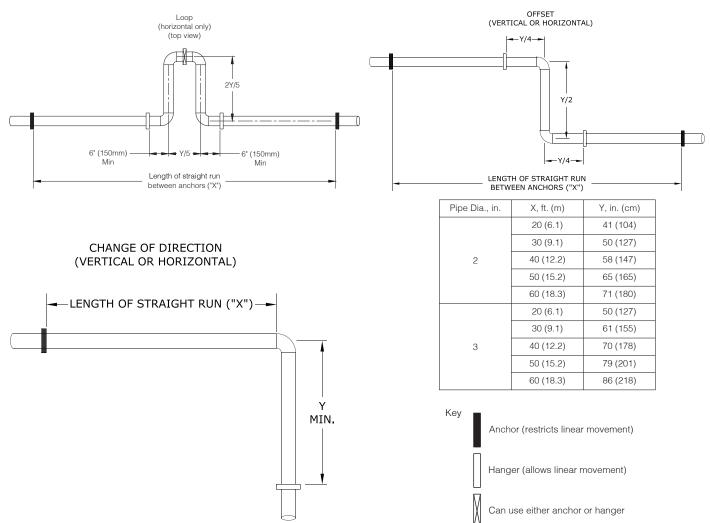
Figure 7-15: CPVC/PVC Venting Expansion Loops
