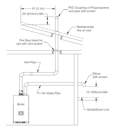
Figure 9-5: Alternate Vertical Vent/Sidewall Air Terminal
