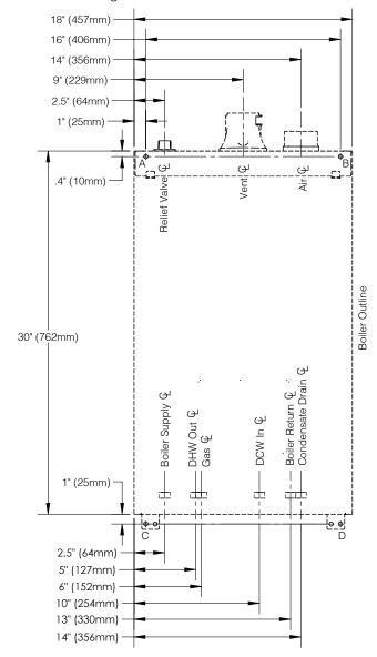
Figure 6-4: Wall Layout and Mounting Holes
