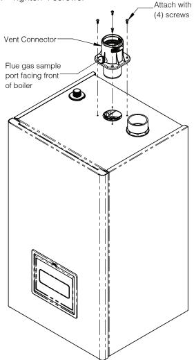
Figure 6-2: Installing Vent Connector
