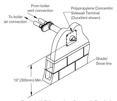
Figure 8-14: Polypropylene Concentric Terminal
