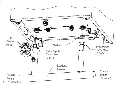
Figure 10-1: Low Loss Header Connections
