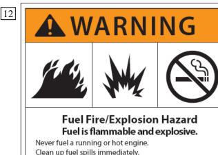
Clean up fuel spills immediately. Ensure there are no fuel leaks before starting. Keep sources of sparks and flames away. Hot exhaust may also ignite spilled fuel. No smoking. Keep a fire extinguisher nearby.
