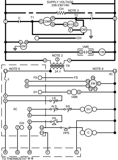
CONTACTOR CRANKCASE HEATER CONDENSER MOTOR HIGH VOLTAGE ČН LOW VOLTAGE FIELD INSTALLED POWER COMP COMPRESSOR EVAPORATOR MOTOR FIELD INSTALLED CONTROL **FUSE** OPTIONAL HIGH VOLTAGE FLAME SENSOR EQUIPMENT GROUND FS OPTIONAL LOW VOLTAGE GND Ġ۷
