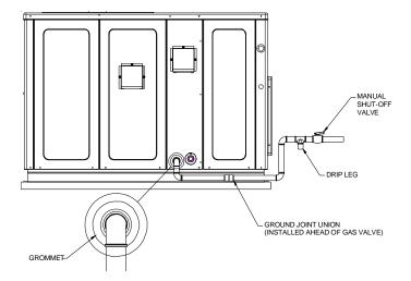
**NOTE:** The unit gas supply entrance is factory sealed with plugs. Keep plugs in place until gas supply is ready to be installed. Once ready, replace the plugs with the supplied grommets and install gas supply line.
