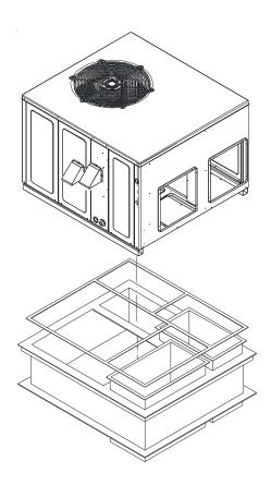
**NOTE:** A roof curb can be used to utilize bottom discharge.
