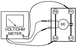
Ohmmeter for testing holding coilVoltmeter for testing contacts
