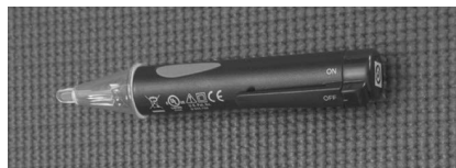
Figure 34 - Non-Contact Circuit Tester
