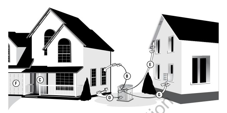
All fossil fuel burning equipment, such as standby generators, contains carbon monoxide (CO) gas in the engine exhaust. CO gas is odorless, colorless and tasteless and is unlikely to be noticed until a person is overcome. CO gas can kill you so it is required that the following is included as part of the installation:
