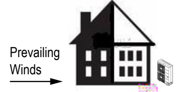
Figure 24: Leeward Side of the Building.
